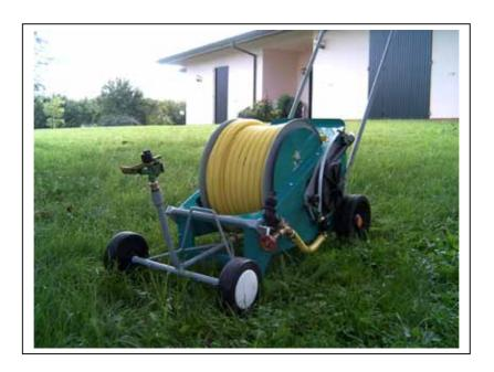
Maintain thin layer on drum gear and on gears near the turbine drive. Drain turbine prior to freezing weather.
