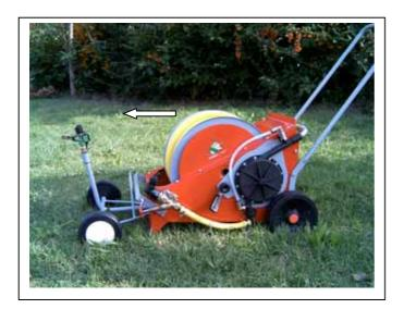
**3.**Pull out the hose perpendicular the machine. Leave always a few wraps on the drum .
