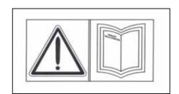
Read this operator's manual before using the machine.
