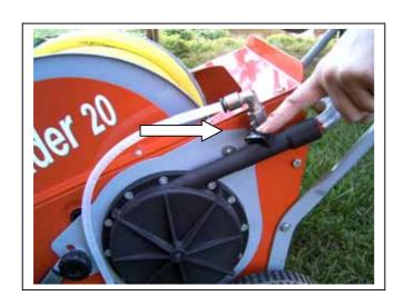
**8.** Adjust speed of cart retraction by turning the ball valve at the turbine. Turning the valve fully closed will increase retraction speed. Opening the valve will slow the retraction rate.
